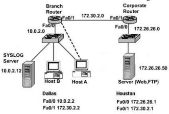
You have been assigned to configure CBAC on a branch router for Certkiller .com. One router from your oil company is named Dallas. The topology is pictured in the graphic. The corporate router has already been configured. All that is left to do is to configure CBAC on the local router to inspect Web and FTP traffic to the corporate server and to allow ICMP from any source to any destination and EIGRP from the
